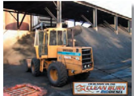
*The Dresser backhoe that is running B20 at UTK. The image in the bottom right is a blow-up of the sticker that is on each side of the vehicle.*
