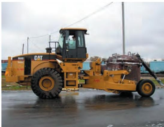
*A crucible carrier transports a load of molten aluminum to the ingot-forming area at the Alcoa South Plant. Alcoa has about fifteen different types of diesel vehicles running B20.*
