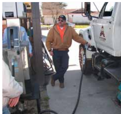
A City of Alcoa fleet driver fills up his vehicle's first load of B20 at the kick-off ceremony. The B20 has a low-NOx additive in it to turn biodiesel's typical small NOx increase into a measurable decrease.
