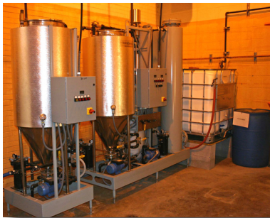
The Biodiesel Logic system that Clarksville has installed has a small carbon footprint. Shown here are the production system, some of the raw materials, and the finished product storage tanks.
