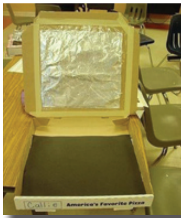
Top - The students had built their own solar ovens using pizza boxes and aluminum foil. Bottom - Couch operates his bicycle-powered generator.
