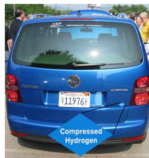
Clockwise from top right: Daimler's F-Cell, Nissan's X-Trail FCV, and Hyundai's Tucson FCV are all fuel cell vehicles and emit only water vapor from the tailpipe. BMW's Hydrogen 7 is essentially a flex-fuel vehicle that uses an internal combustion engine to operate on either hydrogen or gasoline. The Volkswagen Touran HyMotion is also a fuel cell and is shown while refueling at the onsite, mobile refueling station. The fuel cell vehicles all run on compressed hydrogen while the BMW stored its hydrogen on-board liquified -- that is chilled to -423°F.
