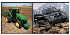
A 7920 John Deere tractor running on B2 and a Jeep Liberty Limited running on B5... biodiesel powered.
