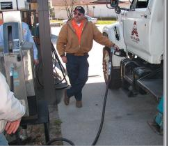
A City of Alcoa fleet driver fills up his vehicle's first load of B20 at the kick-off ceremony. The B20 has a low-NOx additive in it to turn biodiesel's typical small NOx increase into a measurable decrease.
